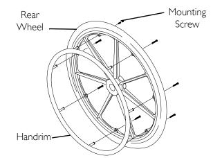
FIGURE 7.2 Replacing Rear Wheel Handrim
